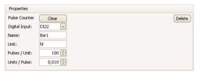
If the name is not defined, the quantity is referenced with its general name *PCxx* (when the *xx* is index corresponding digital input).
