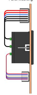
switchobard outer side accessible to laymen minimum protection IP40
