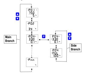
For better orientation, some of parameters (parameter group No. 01, 04, 15) are placed in so called side branches. To enter into a side branch, push P. The dash in the front of the parameter number skips down to the second row indicating the side branch position.
