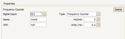
If the name is not defined, the quantity is referenced with its general name FCxx (when the xx is index of corresponding digital input).
