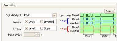
I/O Setup – Standard Digital Output Action Properties
