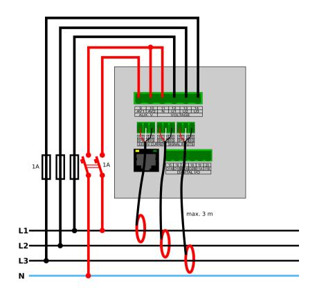
SML133 ... X/5A - Measured Signal Connection Examples
