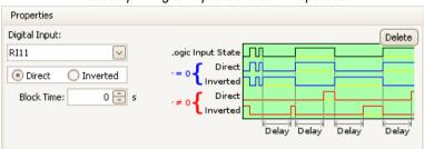
I/O Setup – Digital Input Condition Properties
