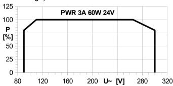
Dependency of maximal power on voltage (for 3-phase AC voltage in case of 1 or 2 lines failure):
