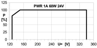
Dependency of maximal power on voltage (for 3-phase AC voltage):
