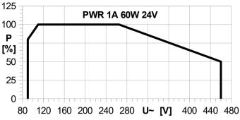
Dependency of maximal power on voltage (DC voltage):
