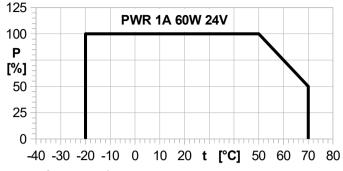
Dependency of maximal load on temperature (for 3-phase AC voltage):
