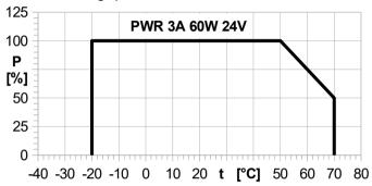
Dependency of maximal power on temperature (for 3-phase AC voltage in case of 1 or 2 lines failure):
