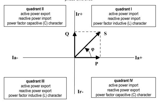
For outright specification of the quadrant, the power factor of the fundamental harmonic component – cos φ – is expressed according to the graph with two attributes:
