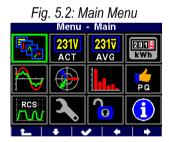
By pressing the \_\_\_\_\_, a *Main menu* window appears. With the \_\_\_\_\_ and \_\_\_\_ you can browse through the menu and select a desired action with the \_\_\_\_\_ or return back using the \_\_\_\_\_ (escape) button.
