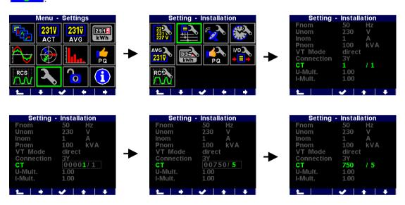
Now you can type new value of the parameter: with the you can move from a digit to another one and to set each digit to target value using the and the parameter is set.
