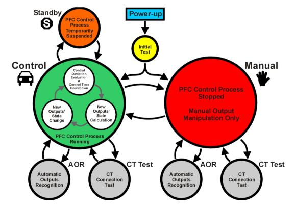
Fig. 4.13: PFC Controller Main Operating States
