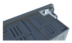
Natural air circulation should be provided inside the distribution board cabinet and in the instrument's neighbourhood no other instrumentation should be installed.
