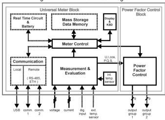
Fig. 1.1: NOVAR 2700 Block Diagram
