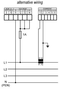
For networks without neutral wire, it is possible to connect all three voltages; then set 1Y3 connection as at previous cases.
