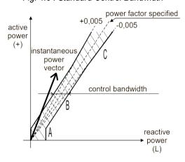
Fig. 4.5: Standard Control Bandwidth
