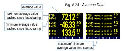
The maximum and minimum registered values can be cleared either manually or automatic clearing can be set.
