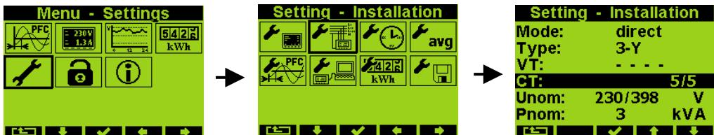
In the window navigate down to the current transformer ratio parameter ( CT ) and choose with the **✓** button.
